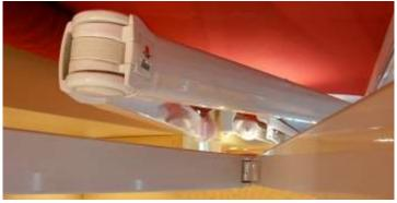
In cases where the total width of the awning does not allow installation of three or more arms, a crossed-arm kit can also be used for one of the arms (always the left-hand arm when viewed from the front). This kit allows an arm to be installed at a lower horizontal level than the others, thereby allowing the arms to cross.
